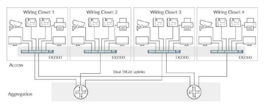
Figure 1: EX2300 switches support Virtual Chassis technology, which enables up to four interconnected switches to operate as a single, logical device.
