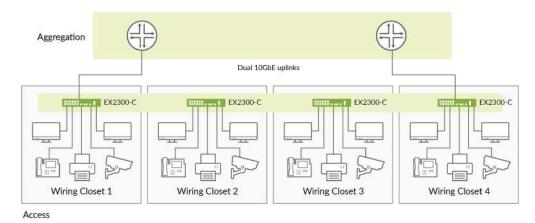
Figure 2: When deployed in a Virtual Chassis configuration, up to four EX2300-C switches can operate as a single, logical device.
